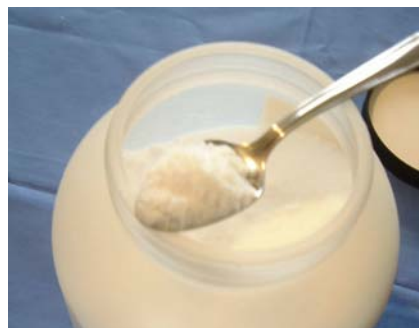
Figure 2: Fumed silica. The small size, hardness and inert nature of silica make it a very versatile and useful material for a wide range of applications and ideal for size analysis by DLS with the SZ-100.
