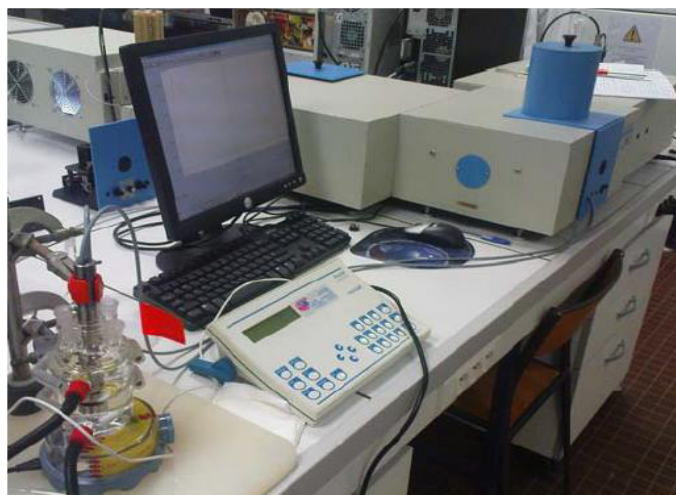
Fig. 3. Experimental set-up for in situ measurements: HORIBA Scientific Fluorolog@-3 in the upper-right corner connected to a Hellma fluorescence probe installed in the reaction vessel in the lower-left corner.
