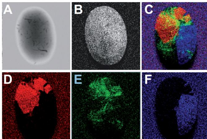
Figure 3: Analysis of ruby (A) x-ray transmission image, (B) chromium XRF image, (C) RGB superimposition of diffraction images D-F, (D) diffraction image 8.68 keV, (E) diffraction image 17.44 keV, (F) diffraction image 10.52 keV
