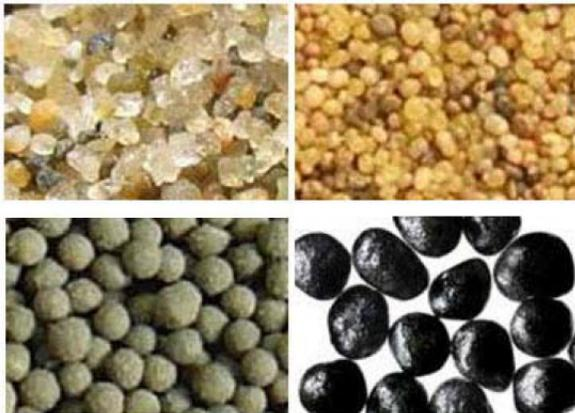
Figure 1: Different types and grades of proppants
