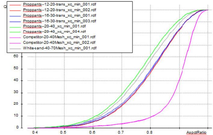
Figure 5: Aspect ratio of the same proppants from the previous figure's size results.
