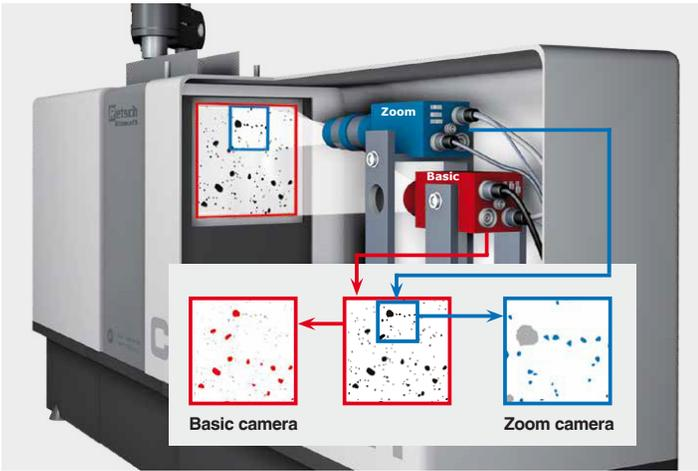
Figure 3: The CAMSIZER Dual Camera Technique
