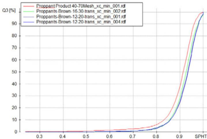
**Figure 7: Shape analysis of the same samples. The blue curve shows the roundest material**
