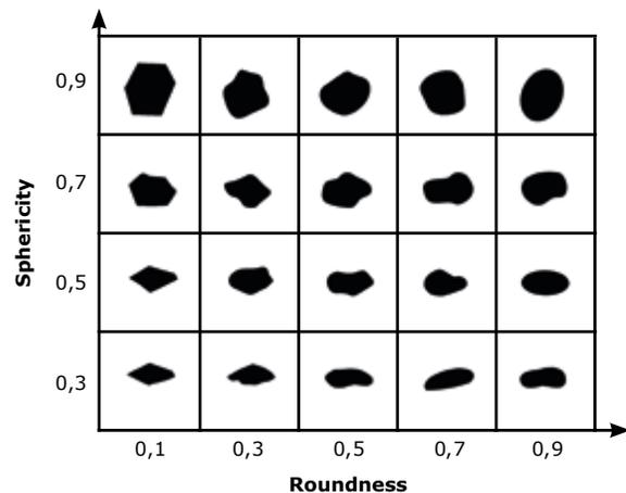
Figure 2: Chart for visual estimation of sphericity (y-axis) and roundness (x-axis)
