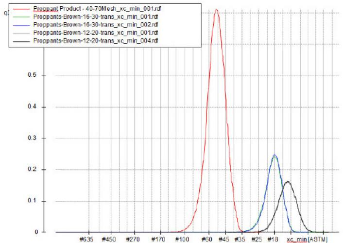
Figure 6: Size analysis of three different products from different suppliers.
