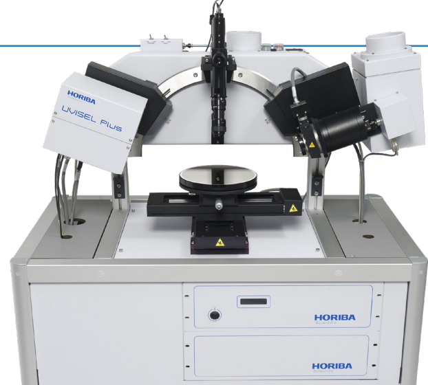
Figure 1: UVISEL Plus spectroscopic ellipsometer equipped with advanced phase modulation and double monochromator system (source: HORIBA)
