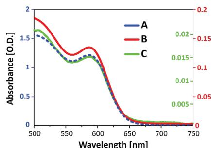
Figure 3: Absorbance spectra for InP\_ZnS Quantum Dots (QDs) at different concentrations
