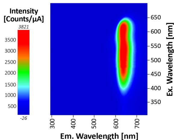
Figure 2: Excitation Emission Matrix (EEM) used to quickly determine optimal spectral ranges for further 2D spectral analysis.
