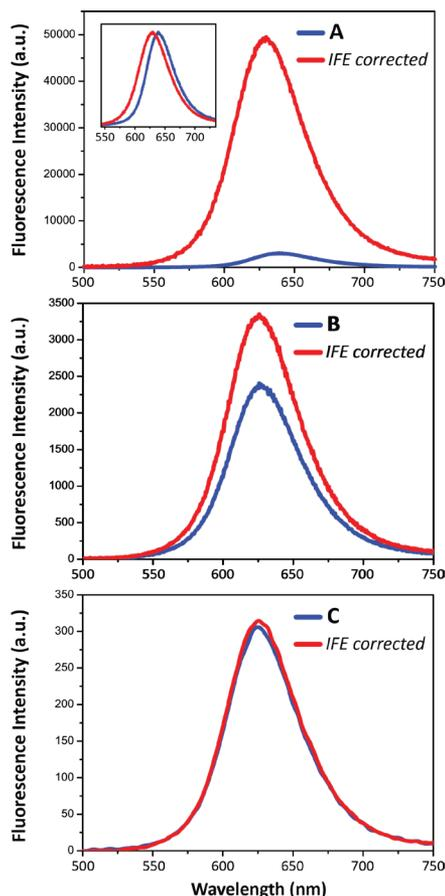
Figure 4: Emission spectra of A (the inset shows the normalized spectra), B and C Quantum Dots (QDs) with and without IFE correction applied.
