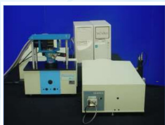
Fig. 1. FluoroLog-3@ system incorporating a closed cycle helium cryostat
