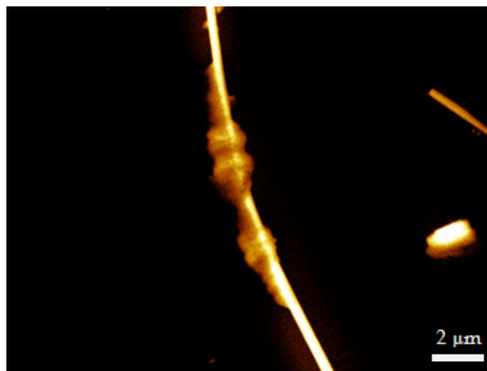
Figure 6: PCL image of a \text{Ga}_2\text{O}_3/\text{SnO}_2 nanowire
