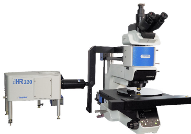
Figure 3: Multi-modal HORIBA SMS system, equipped with motorized X,Y stage for PL mapping, and iHR320.
