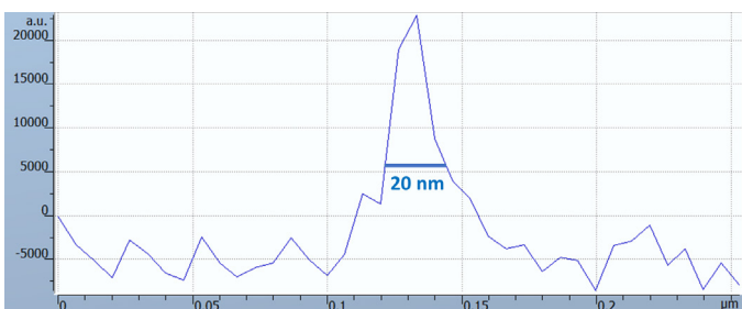
Figure 9: Section analysis of the TERS signal in water (2D band of the CNT) showing a 20 nm TER resolution.
