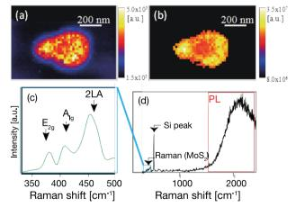
Figure 1: (a) TERS image constructed from integrating signal from 420 to 450 cm<sup>-1</sup>, (b) TEPL image on a single layer MoS<sub>2</sub> flake taken simultaneously, (c) TERS spectrum featuring normal vibration modes:  $E_{2g}$ ,  $A_{1g}$  and 2LA, and (d) full spectrum including TERS peaks and TEPL broad peak.
