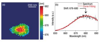
Figure 2: (a) TEPL-shift image and (b) Curve Fitting of PL signal.
