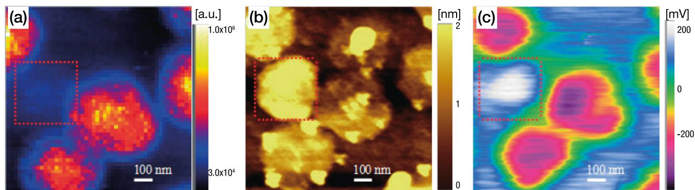
Figure 3: (a) TEPL map, (b) AFM image of monolayer and bilayer  $\text{MoS}_2$  flakes and (c) Kelvin force image (same area as images (a) and (b)).
