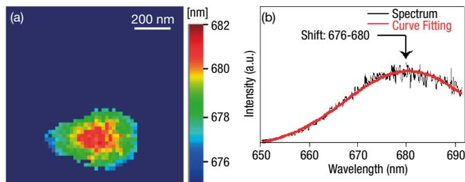
Figure 2: (a) TEPL-shift image and (b) Curve Fitting of PL signal.
