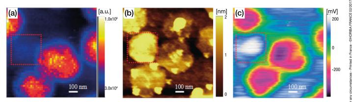
Figure 3: (a) TEPL map, (b) AFM image of monolayer and bilayer MoS<sub>2</sub> flakes and (c) Kelvin force image (same area as images (a) and (b)).
