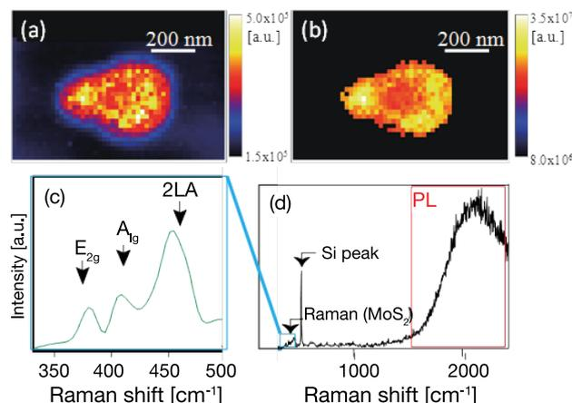
Figure 1: (a) TERS image constructed from integrating signal from 420 to 450 cm<sup>-1</sup>, (b) TEPL image on a single layer MoS<sub>2</sub> flake taken simultaneously, (c) TERS spectrum featuring normal vibration modes: E<sub>2g</sub>, A<sub>1g</sub> and 2LA, and (d) full spectrum including TERS peaks and TEPL broad peak.
