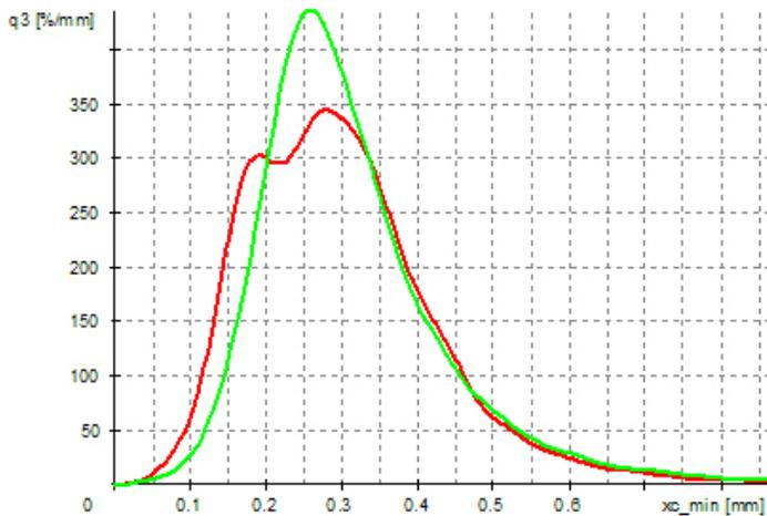
**Figure 2: CAMSIZER XT results for sand used in glass reinforced pipes**
