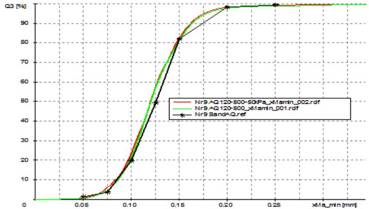
**Figure 3: Size results of sand by sieve and CAMSIZER XT free fall and air jet sampler**
