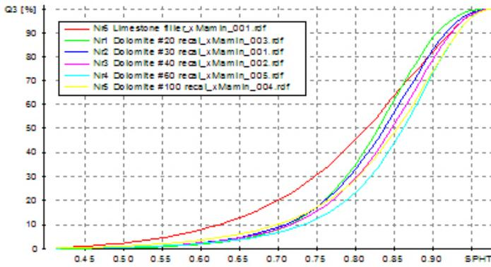
Figure 5 : Sphericity distributions for six grades of limestone
