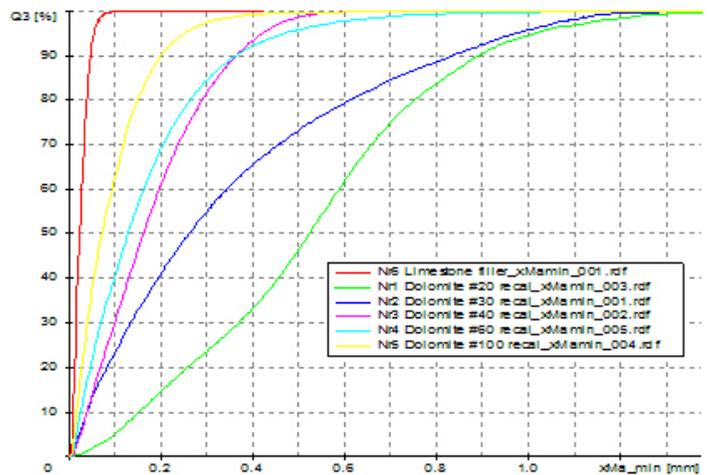
**Figure 4: CAMSIZER XT results for six grades of limestone**
