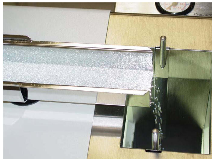
Measurement of glass beads on the CAMSIZER®
