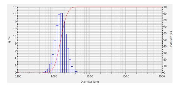
**Asphalt emulsion** Median – 1.56μm D (10%) – 1.02μm D (90%) – 2.40μm Mean – 1.65μm
