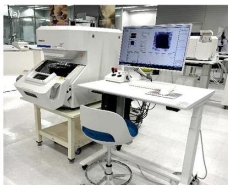
Figure 1. (a) HORIBA XGT-9000 X-ray Analytical Microscope; (b) Schematic diagram of the internal optics; (c) Sample setting on a sample tray.
