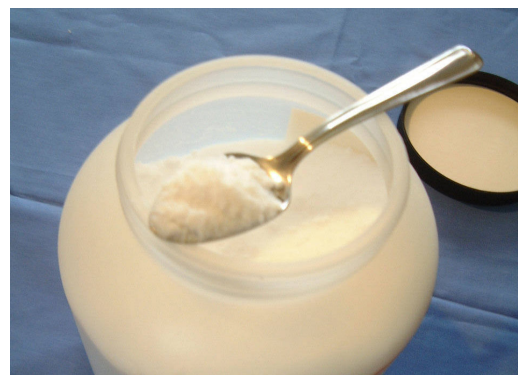
Figure 2: Fumed silica. The small size, hardness and inert nature of silica make it a very versatile and useful material for a wide range of applications and ideal for size analysis by DLS with the SZ-100.
