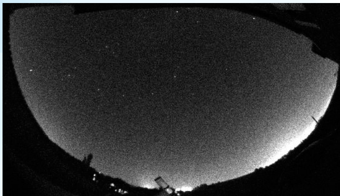
Figure 3: Single 100 ms exposure time, EM gain enabled, fisheye lens ( F = 1.8 mm) with AToR. Magnitude 3 stars can be detected.
