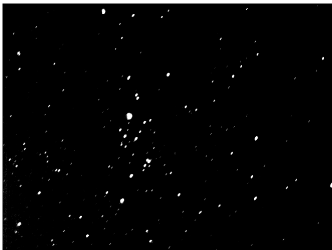
Figure 5: 500 x 50 ms exposure time with no EM gain, 20 mm, f/1 lens with AToR.
