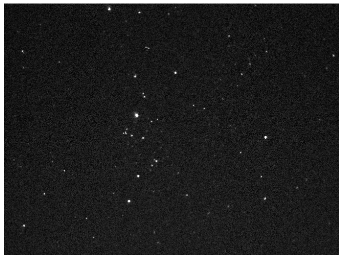
Figure 2: 50 ms exposure time with EM gain enabled. 20 mm, f/1 lens.
