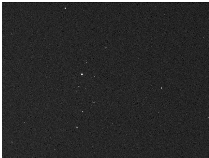
Figure 1: 50 ms exposure time with no EM gain. 20 mm, f/1 lens.
