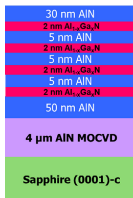
Fig. 2: (left) Structure of Sample, (right) different ratios of Al/Ga in 2 nm AlGaN layer
