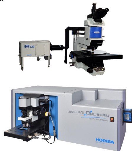
Figure 2. Photograph of the multimodal industrial SMS system (above) and the LabRAM Odyssey (below)
