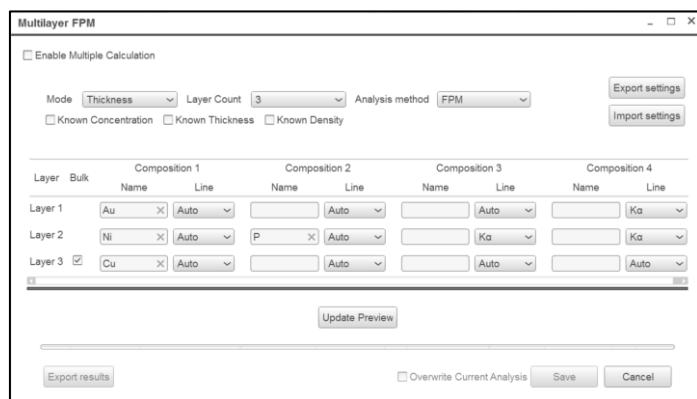
Figure 6. Layer model used for this sample. Standard-less calculation using Multilayer FPM module was applied.
