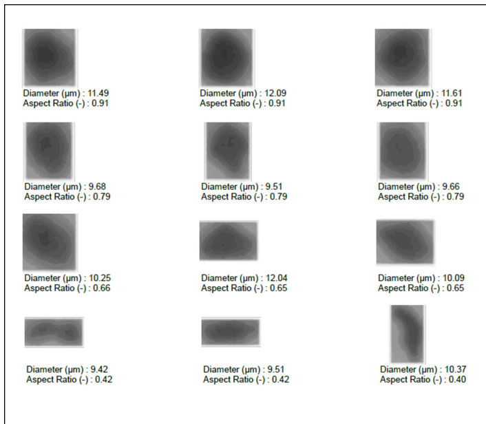
Figure 8. Particle image list for carbon-coated silicon from imaging unit accessory (LY-9610).
