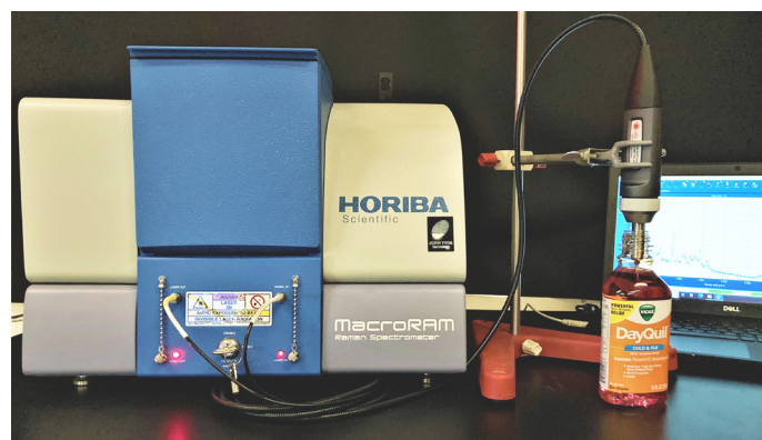
Figure 4: Raman spectra of DayQuil™ and NyQuil™ collected with an immersion probe fiber-coupled to the MacroRAM™ Raman spectrometer, and a picture of the immersion probe setup.
