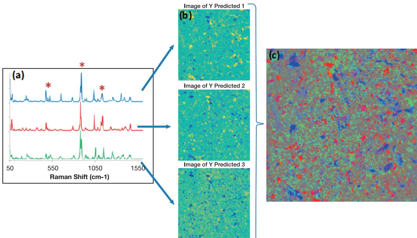
Figure 2: Raman spectrum of  $\alpha$ ,  $\beta$ ,  $\delta$  mannitol (a), distribution maps indicating the spatial distribution of mannitol forms (b) and  $\alpha$ ,  $\beta$ ,  $\delta$  distribution map indicating the composition and the spatial distribution of mannitol forms of a tablet (c).
