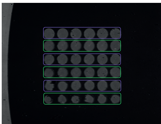
Figure 3: Image of the printed SPRI-Biochip™ CH-LD. Spots of the antibody of interest are framed in purple and negative control spots are framed in green.
