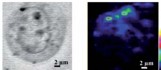
Figure 4: White light image (left) and Raman mapped image showing intensity at 1296-1306  $\text{cm}^{-1}$  (right)
