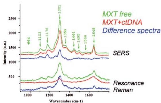
Figure 2: Comparative SERS and resonance Raman spectra of model complexes in solution obtained with 514.5nm excitation. Data have been offset for clarity.
