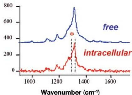
Figure 3: Spectra free and intracellular mitoxantrone. Data have been offset for clarity.
