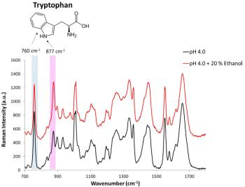
Figure 4: Raman Analysis of lysozyme (200 mg/mL) in 20 mM Citrate-PBS buffer at pH 4.0 before and after the addition of 20 % ethanol. Sample was excited with a 532 nm laser and a grating of 1800 lines/mm on the XploRA, a 200mm focal length instrument.
