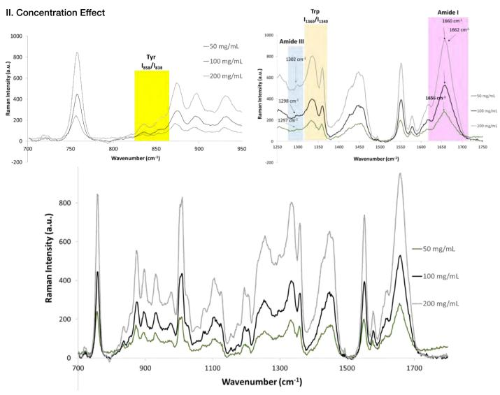
Figure 6: Raman Analysis of lysozyme (200 mg/mL, 100 mg/mL and 50 mg/mL) in 20 mM Citrate-PBS buffer at pH 10.0 . Sample was excited with a 532 nm laser and a grating of 1800 lines/mm.
