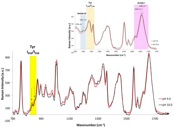
Figure 5: Raman Analysis of lysozyme (200 mg/mL) in 20 mM Citrate-PBS buffer at pH 4.0 and pH 10.0. Sample was excited with a 532 nm laser and a grating of 1800 lines/mm.
