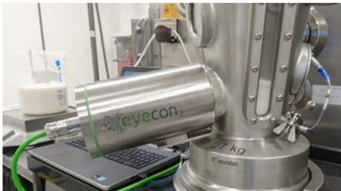
Figure 3. Eyecon 2 in-place on the product container window.
