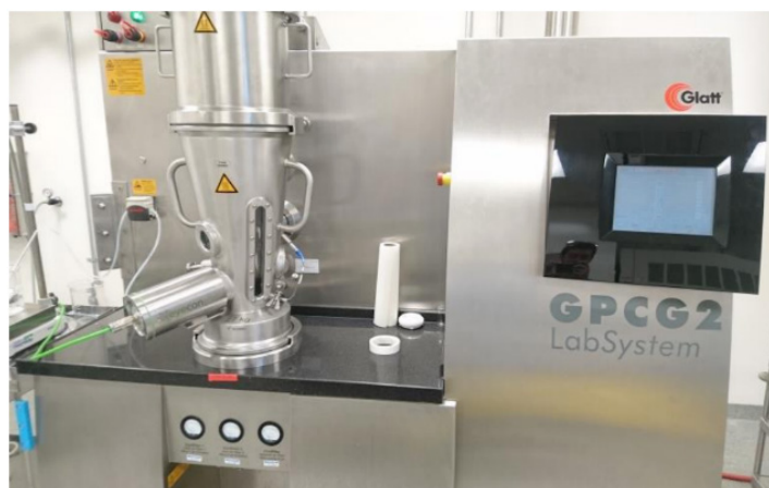
Figure 2. Glatt GPCG2 with Wurster container and Eyecon 2 installed on the left.
