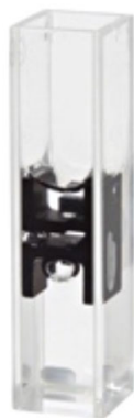
Figure 2. The cuvette includes a black insert that houses a magnetic stir bar to keep virus aggregates particles suspended.
