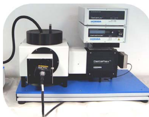
Fig. 2. DeltaFlex with stopped flow accessory entering via a “split” sample chamber lid.
