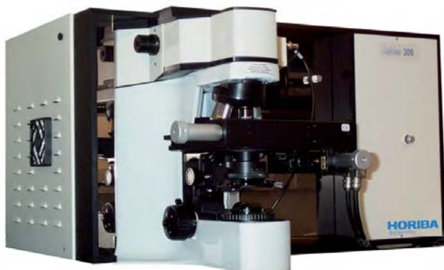
Figure 1: the LabRAM benchtop Raman system
