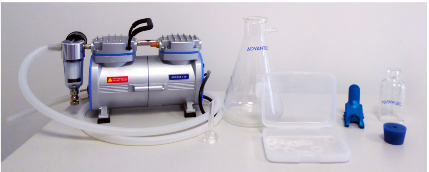
Figure 1: Filtration apparatus: glass funnel, glass support base, silicone stopper, glass flask, and vacuum pump.
