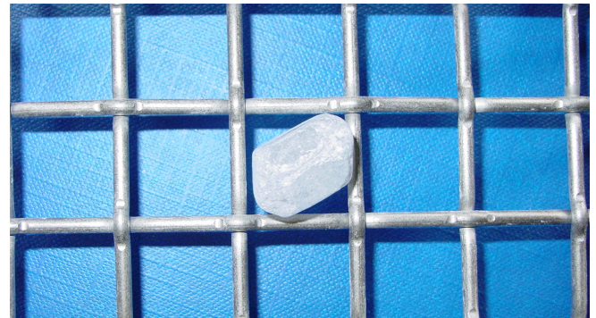
Figure 2. A rectangular shaped sugar crystal compared to the square aperture of the sieve opening
