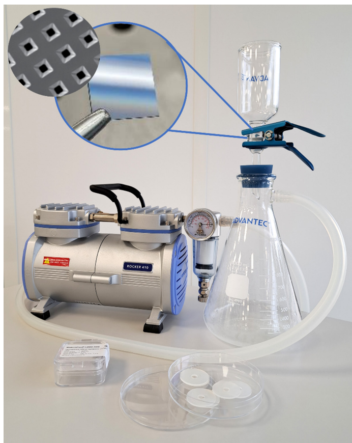
Figure 1. Filtration kit: glass funnel, glass support base, silicone stopper, glass flask, vacuum pump and Si filters (5 \mu\text{m} porosity).
