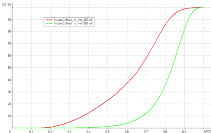
Figure 9: Shape comparison (SPHT) of two different instant coffee products.
