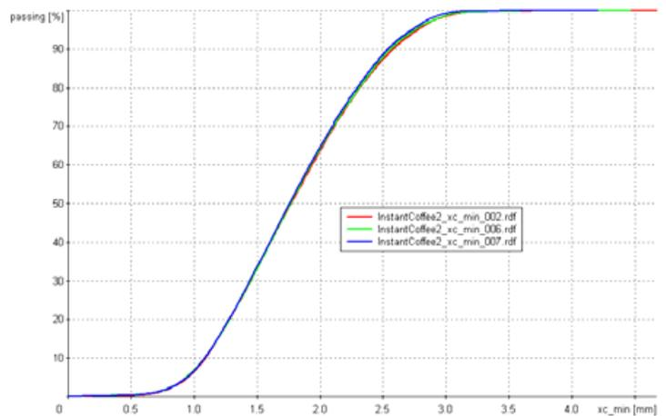
Figure 7: Three different measurements of a single instant coffee product (Precision).
