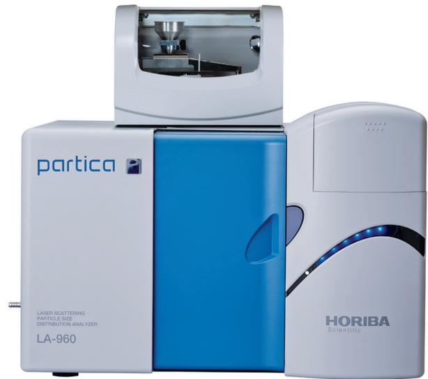
**Figure 3: The HORIBA LA-960 Particle Size Analyzer with PowderJet Dry Feeder accessory.**
