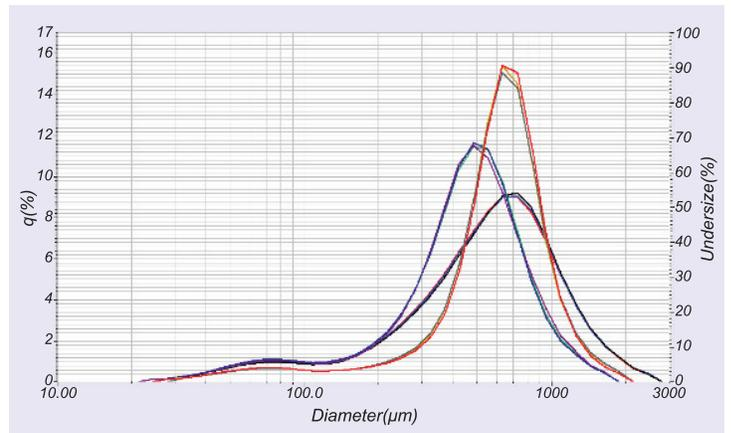
**Figure 5: Nine measurements from nine unique samplings of three different ground coffee products. Notice the excellent repeatability and reproducibility as the three measurements for each product overlay very closely. Notice also the product with coarsest particles greater than 2000 microns.**
