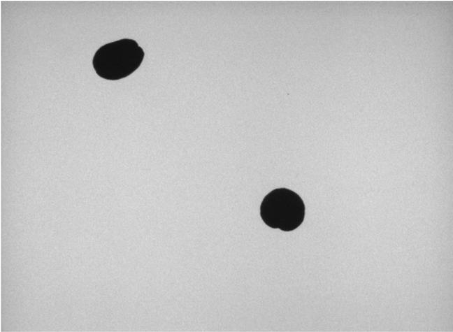
**Figure 2: A captured image from the CAMSIZER showing two green beans (of thousands) measured and classified based on size and shape.**
