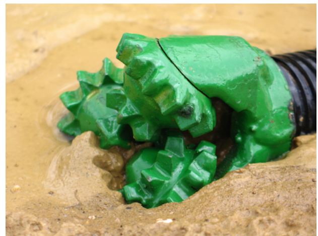
Figure 1: Drill bit in drilling fluid
