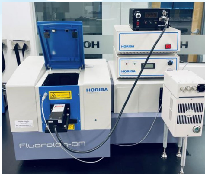
Figure 1. The Fluorolog-QM-LAS shown with sample compartment lid open
