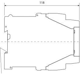
Snap-on mounting on 35 mm DIN rail EN 60715
