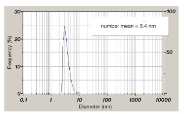
Figure 2: Colloidal platinum particle size result
