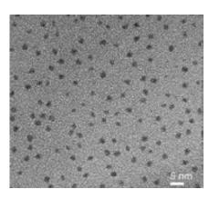
Figure 1: TEM photograph of colloidal platinum suspension\*
