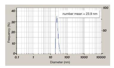
Figure 2: Colloidal copper particle size result
