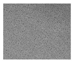
Figure 1: TEM photograph of colloidal copper\*
