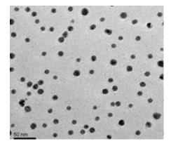
Figure 1: TEM photograph of colloidal silver suspension\*
