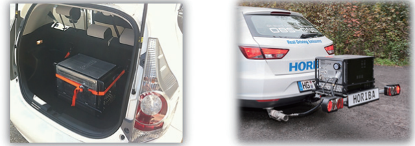
Figure 2 Installation of PEMS on the vehicle
