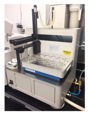
Figure 2. LA-960V2 Slurry AutoSampler
