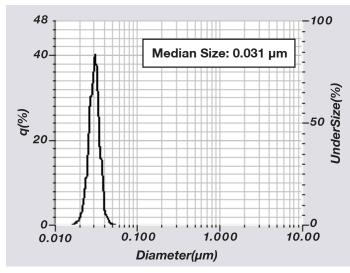
Figure 1: LUDOX TM-50 particle size distribution.
