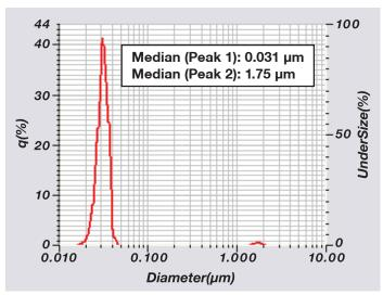
0.05wt% Geltech 1.5 in LUDOX TM result shows both oversize particle detection and very good accuracy for both components.
